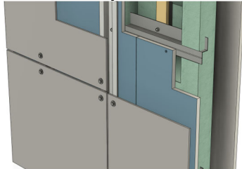
Figure 1: Back-Lattice sm places the thermally broken structural, thermal, and vapor control layers directly inward of the air and water-protected sheathing.
